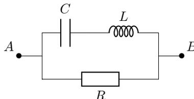
a)  $Z_{AB} = \dots\dots\dots$
